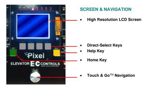
Figure 1.4.2 - Pixel Screen & Navigation
