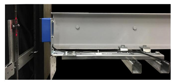
Figure E1.7: CEDES APS Camera Mounting Bracket
