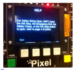
Press the yellow HELP button and details about how to resolve the fault are displayed.
