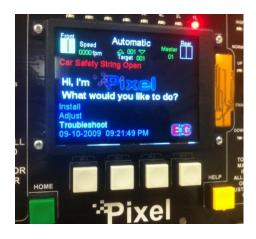
Pixel home screen displays **Car Safety String Open** Fault (shown in red).
