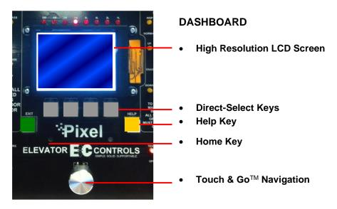
Figure i1 - System Access Point
