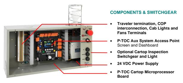
Figure 1.3.2 - Typical Pixel Cartop Interface
