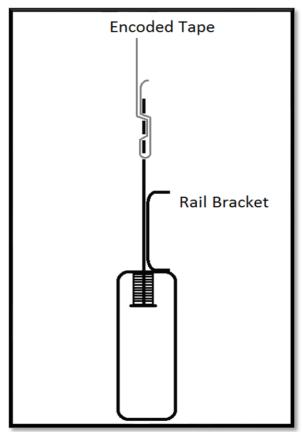
Figure E1.5: Encoded Tape connection.
