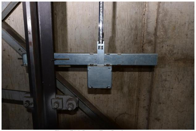
Figure E1.4: Bottom Tape Bracket
