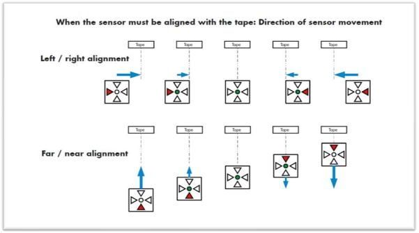
Figure E.1.9: Camera Sensor Alignment
