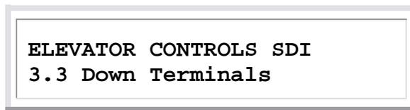
Press SELECT on the Down Terminals submenu, shown above, to view the status of the down terminal slowdowns. Please refer to Appendix A-Drawings SDI 7D for a more detailed description of how to select Submenu 3 items.
