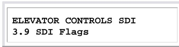
Press SELECT on the SDI Flags submenu, shown above, to view the status of the SDI flags communicated to the elevator microprocessor. Please refer to Appendix A-Drawings SDI 7D for a more detailed description of how to select Submenu 3 items.
