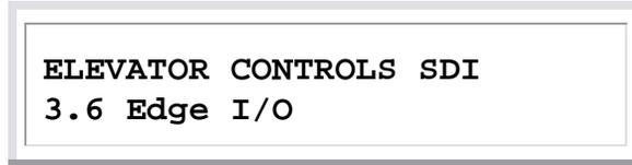
Press SELECT on the Edge I/O submenu, shown above, to view the status of the edge inputs and outputs. Please refer to Appendix A-Drawings SDI 7D for a more detailed description of how to select Submenu 3 items.
