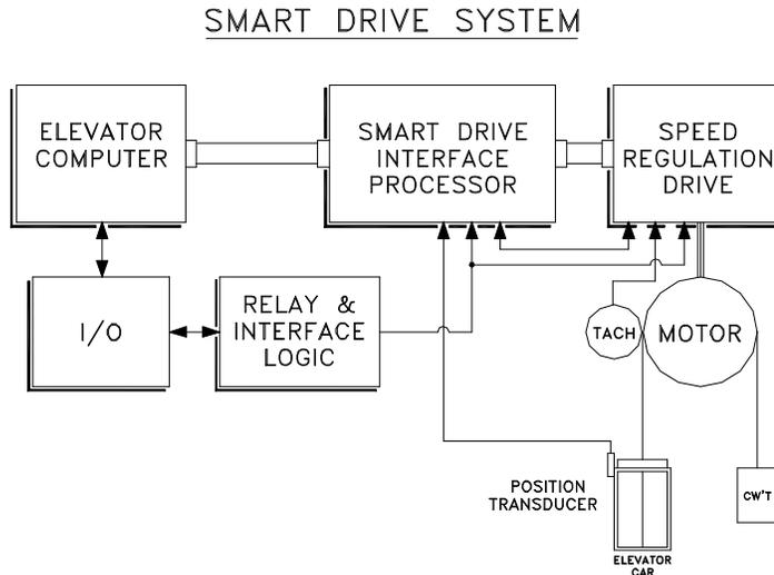
1. Elevator Car Controller Computer. It controls all of the elevator sequencing and signals. The elevator computer is the master computer, and tells the Smart Drive Interface (SDI) and the Speed Regulator what to do.
